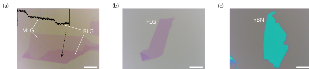
Figure 3.5: Examples of ideal flakes for heterostructures (scale bars: 20 \mu\text{m} ). (a) Contrast-enhanced optical image of monolayer and bilayer graphene present within the same flake. Inset: Profile of the greyscale pixel intensity along the dashed arrow. (b) \sim 3 nm few-layer graphite (FLG) flake. (c) \sim 42 nm hexagonal boron nitride (hBN) flake. The thicknesses of FLG and hBN flakes are determined using atomic-force microscopy.
